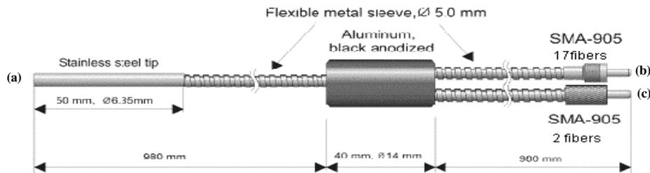
Figure 2. Fiber optic probe: (a) the probe consists of 19 fibers of 200  $\mu\text{m}$  diameter, (b) 17 fibers carry light to the samples, and (c) and two fibers carry radiation back from the sample to the spectrophotometer.
