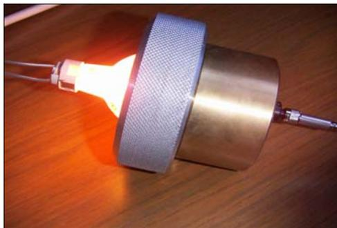
Figure 1. Metal holder for the lamp and the fiber optic probe.
